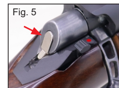
Cocking indicator on "fired" position
